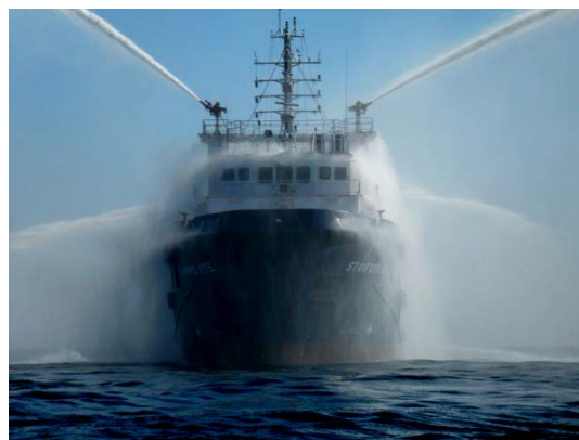
Figure 3: Fire-Fighting System under operation
