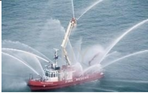
Figure 4: Marine External Fire Fighting System under operation
