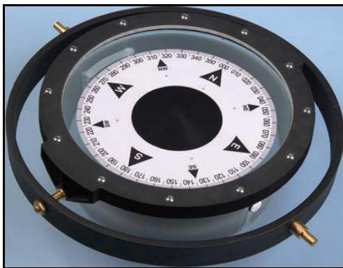
Figure 1 A magnetic rose of MK 2000S Compass Outfit 1
