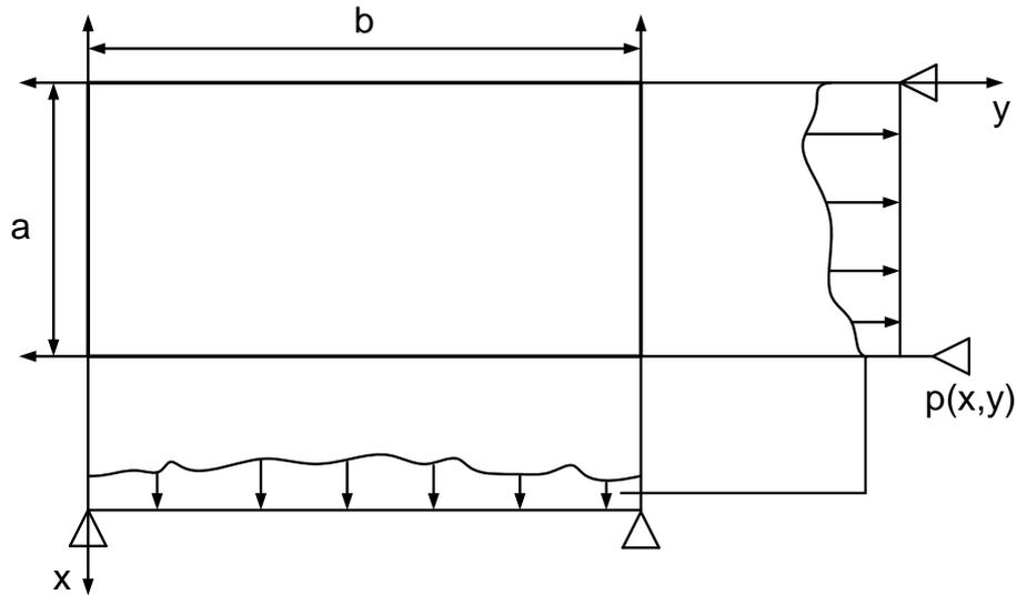
**Figure 3. The plate simply supported loaded with  $p(x)$  varying on the direction**
