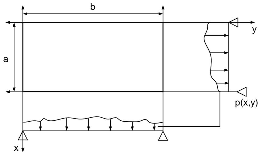
**Figure 4. The plate studied with symmetry planes and coordinate system of axes.**
