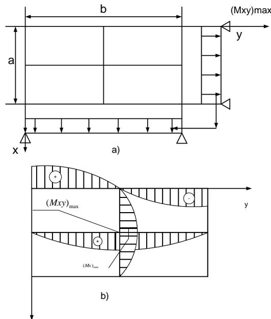
**Figure 2. The rectangular orthotropic plate loaded with a normal load uniformly distributed**
