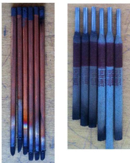
Figure 7. Cutting (left) and gouging (right) electrodes after experiments
