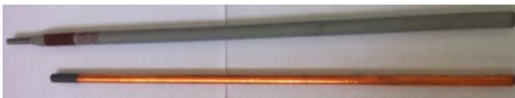
Figure 2. Cutting (lower) and gouging (upper) electrodes before experiments
