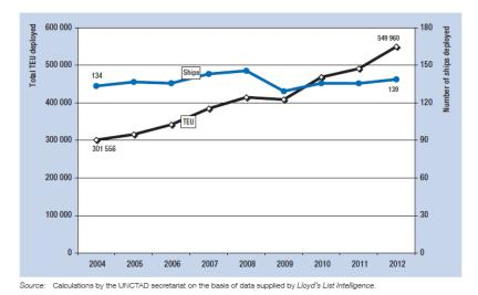
Figure 7. Trends in container-ship fleet deployment: number of ships and their total TEU carrying capacity
