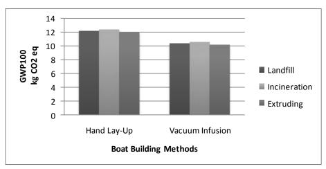
Figure 3 Comparison of GWP<sub>100</sub> results between hand lay-up and vacuum infusion method
