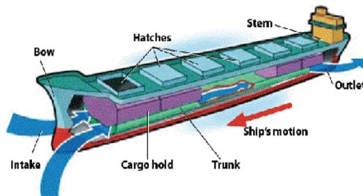
Fig.1. Ballast Free Concept [Source: 6]
