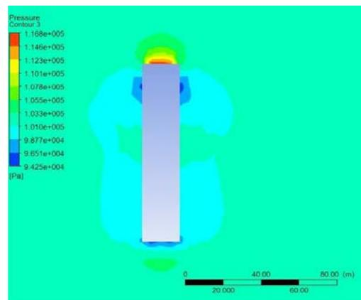
Fig. 10. Ansys pressure results on XOZ plane
