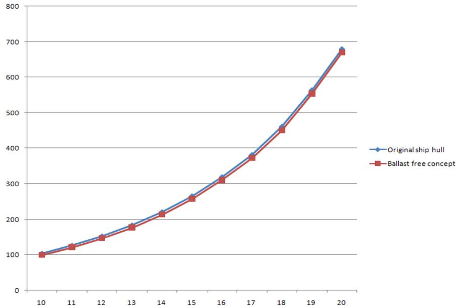
**Fig.12. Resistance versus speed for original shape(blue) and for the studied concept(red)**
