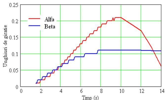
Fig. 2. The time variation of attack angle ( $\alpha$ ) and drift angle ( $\beta$ )
