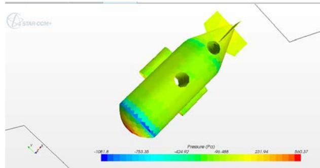
Fig. 5 Pressure distribution on ROV body for 2 m/s speed
