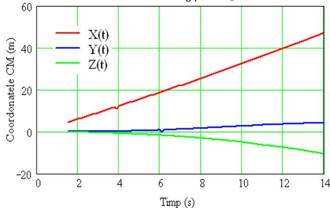
**Fig.1. The mass center coordinates, in fixed reference system.**
