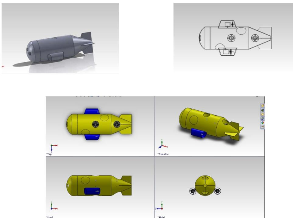
Fig. 3 Sketches and views of ROV prototype
