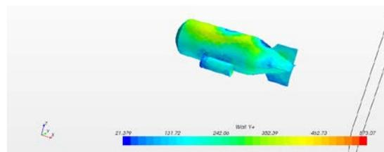
Fig. 7 The horizontal component of drag force and Reynolds numbers distribution, ROV is going to surface at 30 degrees angle and drifting to right, 0,433 lateral speed, 0,968 horizontal speed, 0,5 ascensionspeed,  $F = -19,639\text{ N}$
