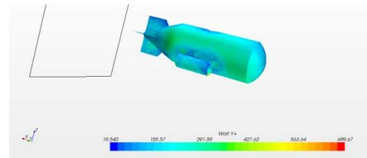
Fig. 6 The vertically component of drag force and Reynolds numbers distribution, ROV is going to surface at 30 degrees angle, 0,866 horizontal speed, 0,5 m/s ascension speed,  $F = -94,128\text{ N}$
