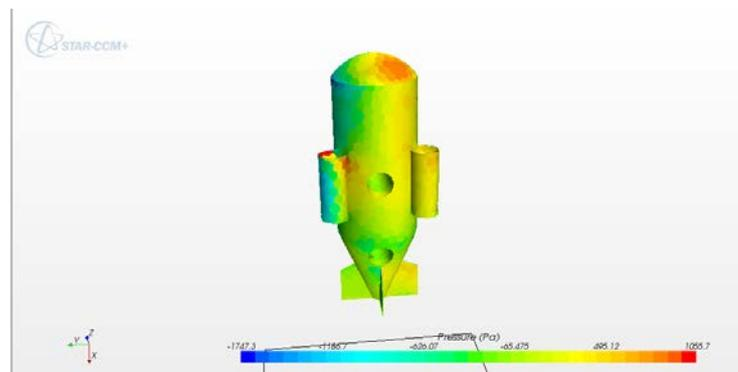
Fig. 8 Pressure distribution on ROV body for the same conditions as in Fig.6 (bellow view)
