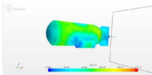
Fig. 4 The drag force and Reynolds numbers distribution for 2 m/s speed,  $F = -65,94\text{ N}$
