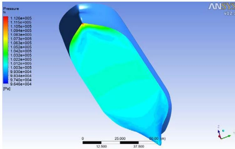
Figure 6. Pressure variation on the ship's hull
