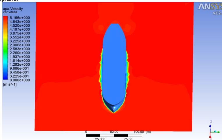
**Figure 4. Velocity variation on the free surface plane**
