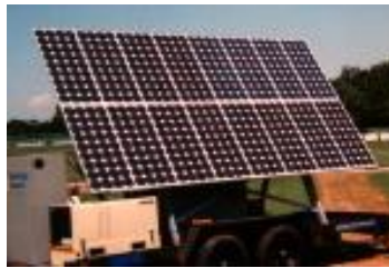
Autonomous hybrid system with photovoltaic panels (Photo: DIERET Course)
