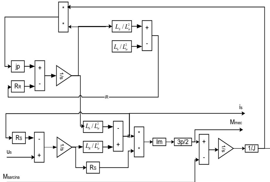
Fig.2 Block scheme for an asynchronous machine with voltage plugging,  $\alpha\beta$  representation
