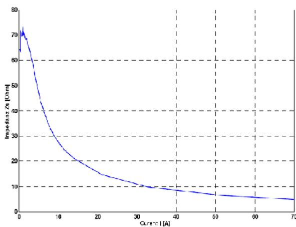
Fig.5 Impedance depending on current
