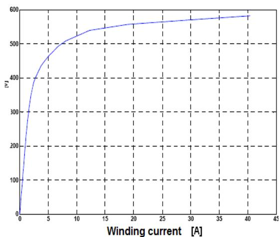
Fig.4 Magnetization diagram
