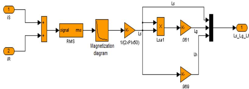
**Fig.7 Implementing inductance dependence on magnetization current**
