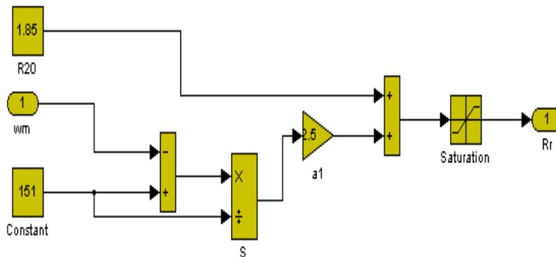
**Fig.10 Rotor resistance variation with slide implemented in Matlab – Simulink**
