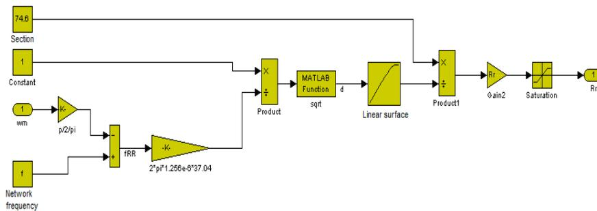
**Fig.9 Pelicular effect is supporting the rotor resistance**
