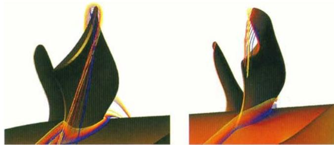
Figure 6: Comparison of two geometrical variations of blade tip with calculated streamlines (FENFLOSS)
