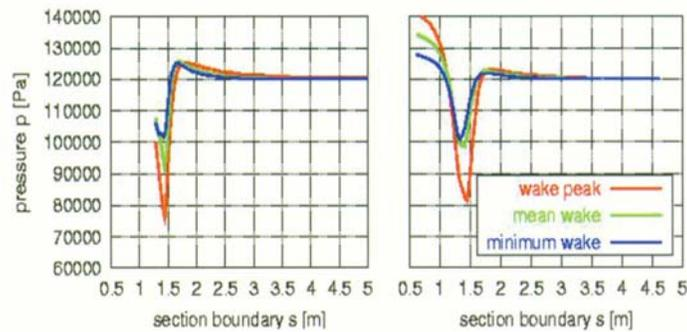
Figure 7: Comparison of the calculated pressure distribution behind the propellers for both geometries (FENFLOSS)
