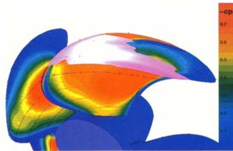
Figure 4: Calculated developed cavitation (PUF-3A)
