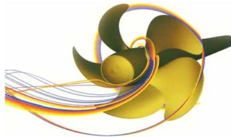
Figure 1: Escher Wyss Controllable Pitch Propellers with calculated streamlines
