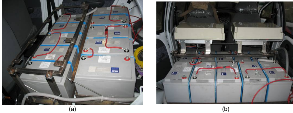
Fig. 4 The battery package (a) and the power modules mounted on top of it (b)
