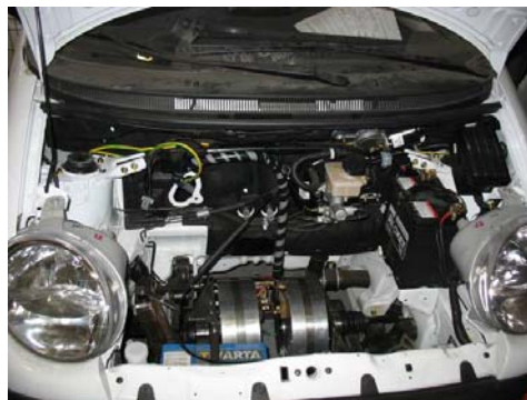
Fig. 7 The independent wheel drive, with two brushless DC motors
