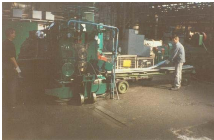
Fig. 2. Lamination Plant of Plated Ingots
