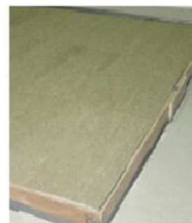
2x 50 mm Rockwool Marine Slab 80 during testing of absorption value
